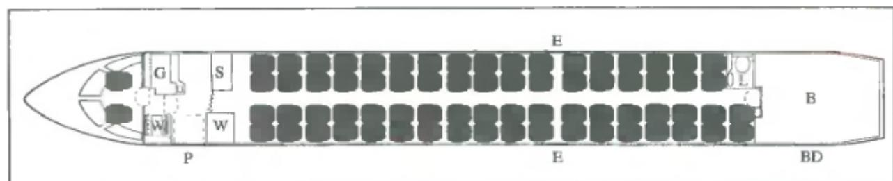
Typical CRJ700 seating plan for 70 passengers at 79 cm (31 in) pitch, with 15.7 m<sup>3</sup> (555 cu ft) of baggage
